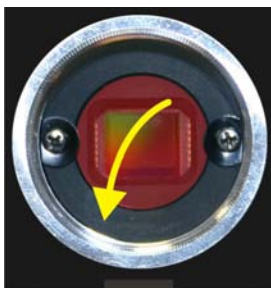
Figure 240: Cleaning fixed uEye filter glasses
