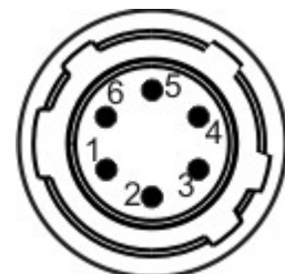
Figure 273: GigE uEye SE - Hirose connector male, camera rear view
