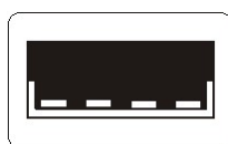
Figure 93: USB standard-A socket (four pins)
