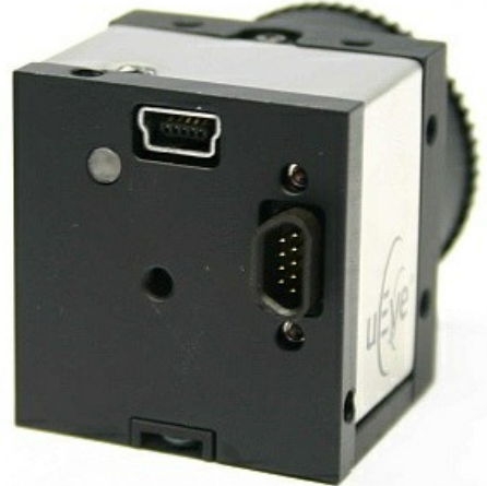
Figure 14: USB uEye SE revision 2.0 (red/green LED)
