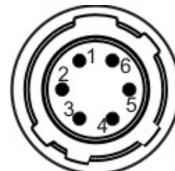
Figure 249: USB uEye ME - Hirose connector, camera rear view
